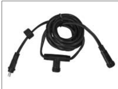
HARNESS2-OD 2-Light Harness 92" Plug-in lead 18AWG IP65 (Waterproof connectors) Fixture Spacing: 46"; Lead: 46"
