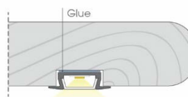
G Recessed Mounting into a Mitered Groove using a flanged Channel
