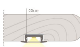
G Recessed Mounting into a Mitered Groove using a flanged Channel
