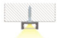
D Surface Mounting with Bracket
