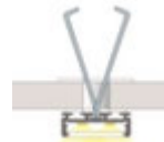
G Recessed Mounting into a Mitered Groove using a flanged Channel
